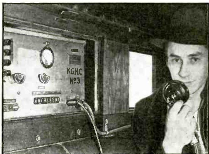
STATION KGHC is a 10-W. mobile unit located in the cab of a rotary snow-plow operating in the Snoqualmie Summit area. A battery-operated 12-V. dynamotor supplies the transmitter's power. The receiver is a police-type superhet.
